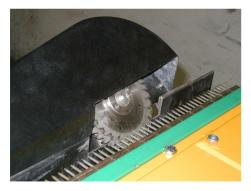
The notching is adjustable in depth according to size of the tobacco feet.
