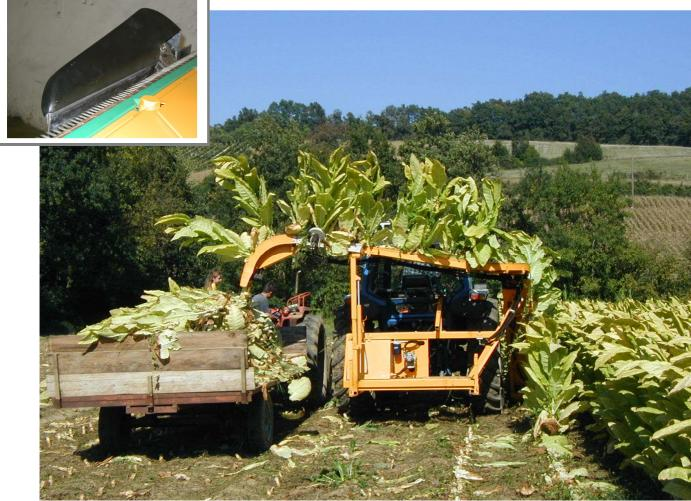
The burley tobacco harvester enable the cutting of 1800 to 2200 stalks/hour, the notch on the stalk and the automatic loading on the trailer, without manual intervention.
