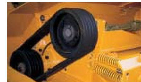
Transmission: double drive and automatic belt tension.
