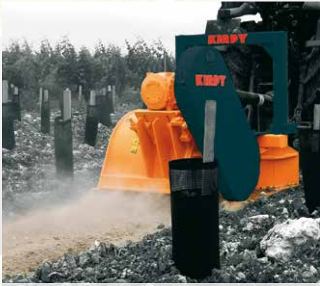
KIRPY BP 65/14 stone crusher working with 3-point vineyard tractor
